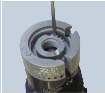
Grinding electrodes: - 4 different angles, 6 different electrode diameters
