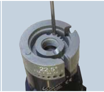
Grinding electrodes: – 4 different angles, 6 different electrode diameters
