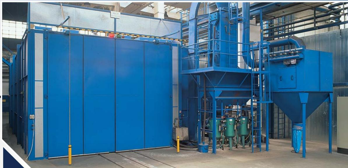
Multi-funnel blasting chamber with magnetic separator suitable for use with metallic or non-metallic abrasives for blasting of conventional structural steel, alloy and stainless steel. ▲
