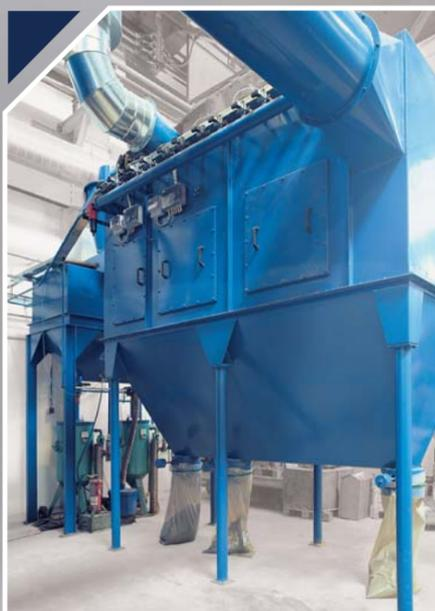
Special mobile multi-funnel trolley design eliminating the possibility of soiling the surrounding of the equipment by the abrasive while unloading or handling the processed components in front of the chamber. ▲
