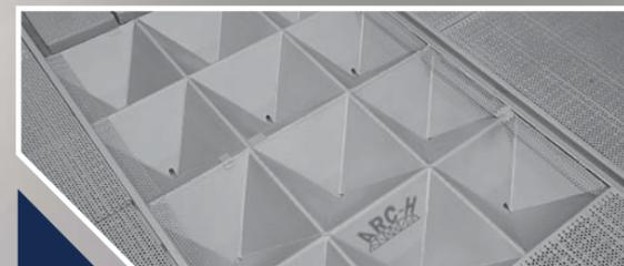
Special multi-funnel floor used for drawing-off the abrasive and its consequent recycling. ▲
