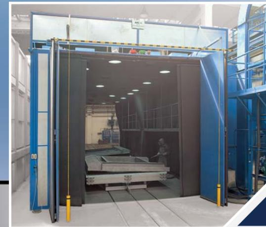
Mobile trolleys driven by an under-surface chain conveyor. One trolley is equipped with a turning table. ▲
